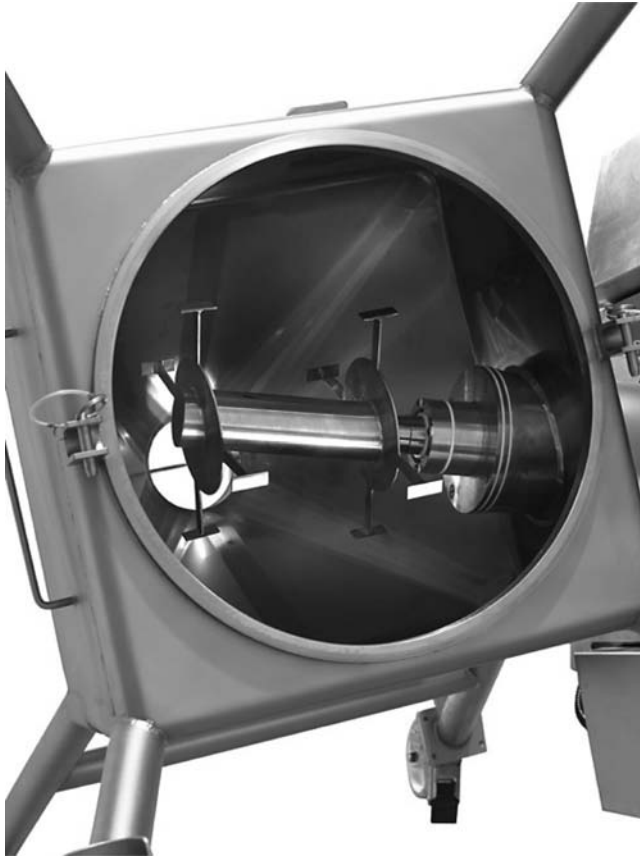
Figure 7.6 Tumbling bin blender with an intensifier bar. (Courtesy of Patterson–Kelley Co., Pennsylvania.)
