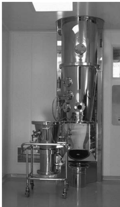
Figure 4.1 Top spray fluidized bed granulator.
