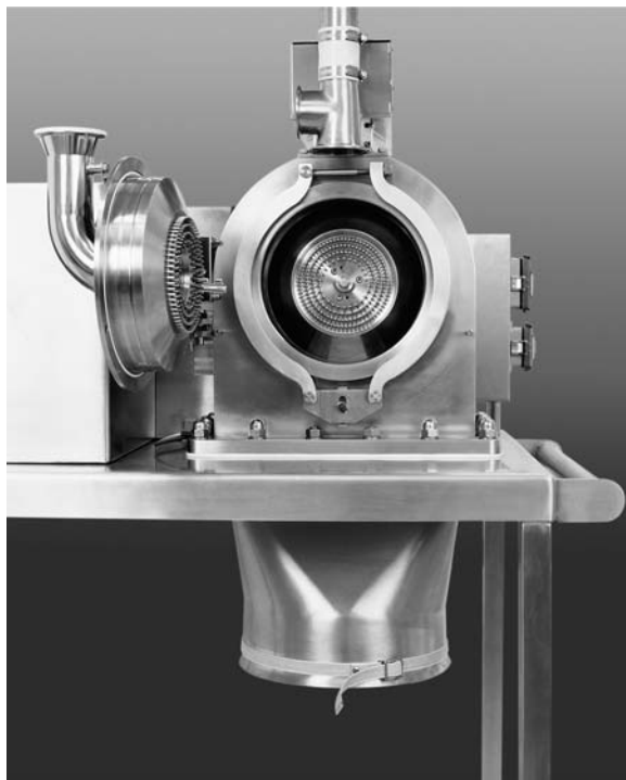
Figure 8.1 Pin mill internals. (Photo courtesy of Hosokawa Micron Powder Systems.)
