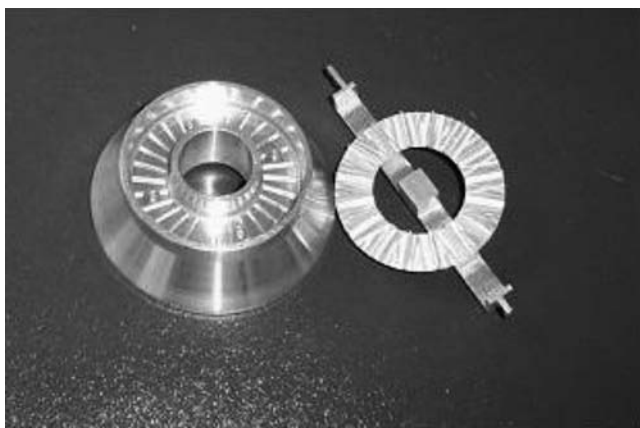
Figure 7.4 Schulze ring shear tester annular trough.
