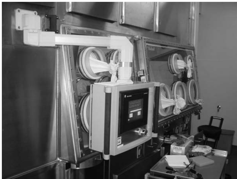
Figure 17.3 Isolator with multiple glove ports in different sizes.
