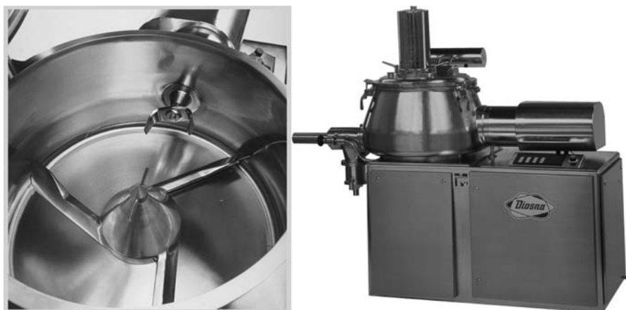
Figure 5.1 Diosna P-150 Granulator. The unit is shown on the right, and the inside of the granulator bowl on the left showing the impeller blade and the chopper.
