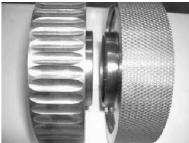
Figure 6.2 Dry granulation roll design options: briquetting (left) and continuous ribbon (right).
