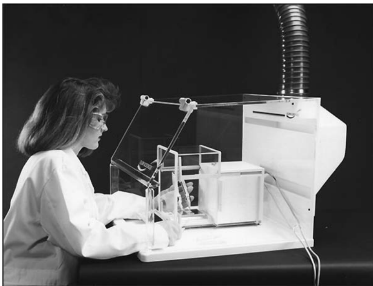
Figure 16.2 An example of a ventilated weighing enclosure.
